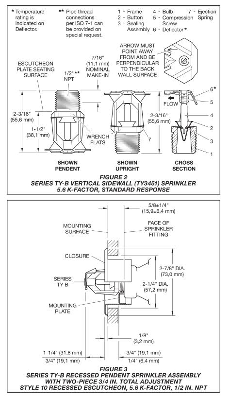
A leak-tight 1/2 in. NPT sprinkler joint should be obtained by applying a minimum-to-maximum torque of 7 to 14 lb-ft (9,5 to 19,0 N·m). Higher levels of torque may distort the sprinkler inlet and cause leakage or impairment of the sprinkler. Do not attempt to make-up for insufficient adjustment in the escutcheon plate by under- or overtightening the sprinkler. Readjust the position of the sprinkler fitting to suit.
