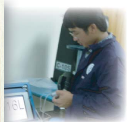
Positive Material Identification Incoming materials are positively identified to verify conformance to Al-Iman's PURCHASE ORDER SPECIFICATION.
